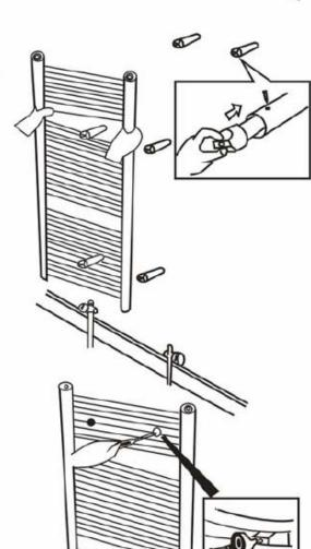
7 Offer the ladder rail A up to the fixing brackets and place bolt J through the bracket bush K.
