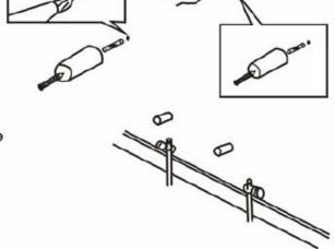
6 Place the spacer H inside the wall support and insert the small screw G into the hole in the wall support. Don't over-tighten to allow for adjustment later.
