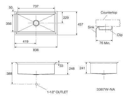
All measurements shown are in millimetres.
