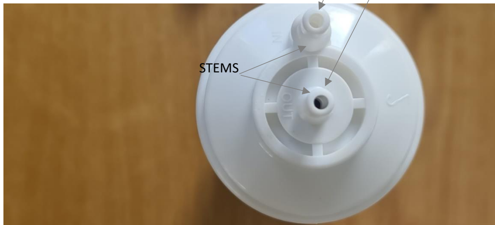
Figure 5. Push smaller diameter of elbow push fit fittings fully on to the IN and OUT stems of the filter (will feel click when fully inserted into position on the filter) as shown below
