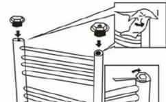
3 Thread the tails from the valves (not supplied) into the bottom two threads. Apply PTFE tape.
