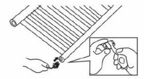
4 The wall supports should be fitted at approximately 10cms from the inside edge of the ladder rail - 2 near the top of the ladder rail and 2 near the bottom.
