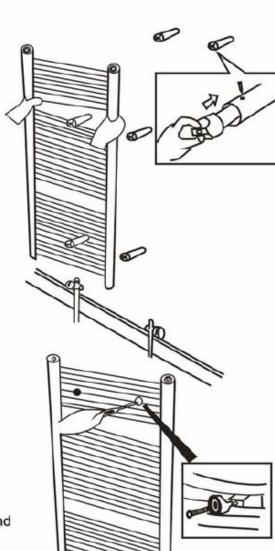
7 Offer the ladder rail A up to the fixing brackets and place bolt J through the bracket bush K.
