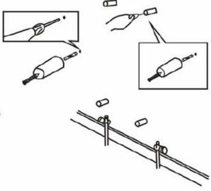
6 Place the spacer H inside the wall support and insert the small screw G into the hole in the wall support. Don't over-tighten to allow for adjustment later.
