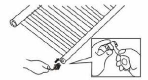
The wall supports should be fitted at approximately 10cms from the inside edge of the ladder rail - 2 near the top of the ladder rail and 2 near the bottom. The mounting height can be varied between any of the ladder rail bars to allow for finding the best fixing point on the wall. Mark the fixing points with a pencil.
